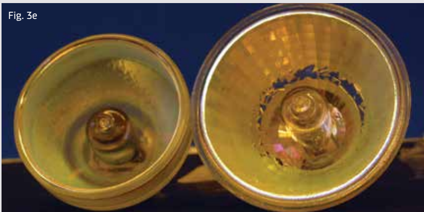
Examples of LCUs where the optics have become damaged: overheated LED, causing bubbles and yellowing in the LED chip (Figs. 3a, 3b); damaged or contaminated light tips (Figs. 3c, 3d); and reflector damage (Fig. 3e).
