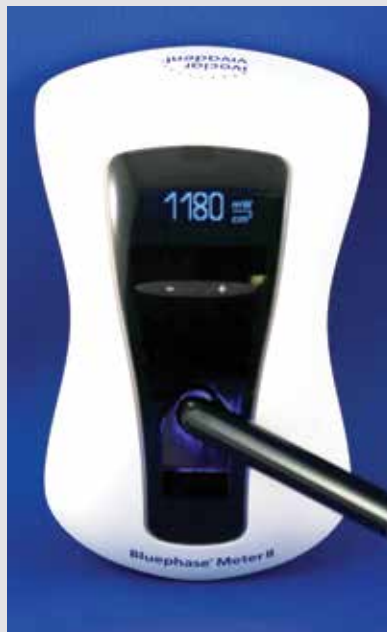
Figs. 5a–b: The Bluephase Meter II, showing the tip diameter guide on the back of the radiometer and the irradiance recording
