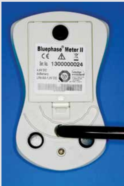
Figs. 5a–b: The Bluephase Meter II, showing the tip diameter guide on the back of the radiometer and the irradiance recording
