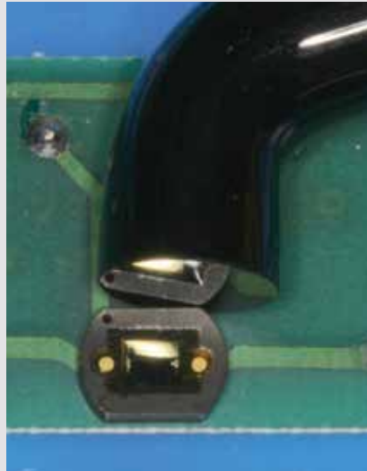
Fig. 4b: Light tip in relationship to sensor size used in radiometer
